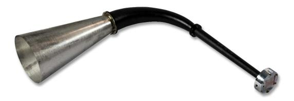
ACS acoustic cleaners use compressed air to flex a titanium diaphragm to produce pressure pulses that are amplified by the bell. The resulting low frequency/high energy sound waves that are emitted resonates/dislodges particulate deposits. The displaced particulate deposits are then removed by gravity and/or gas flow.
